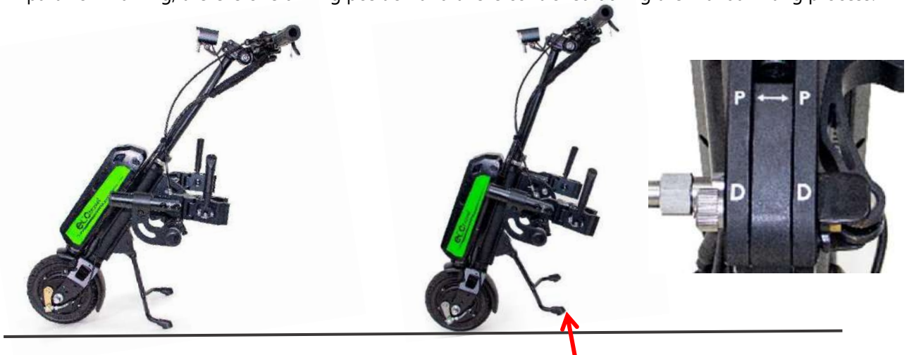
Figure 25. Parking-P (1), and Drive-D (2) Positions for Manual Clamp/Lift Devices
