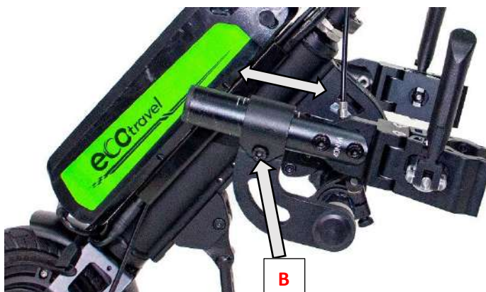
Figure 22. Showing the Depth Adjustment of the Clamp Mechanism in Relation to the Device
