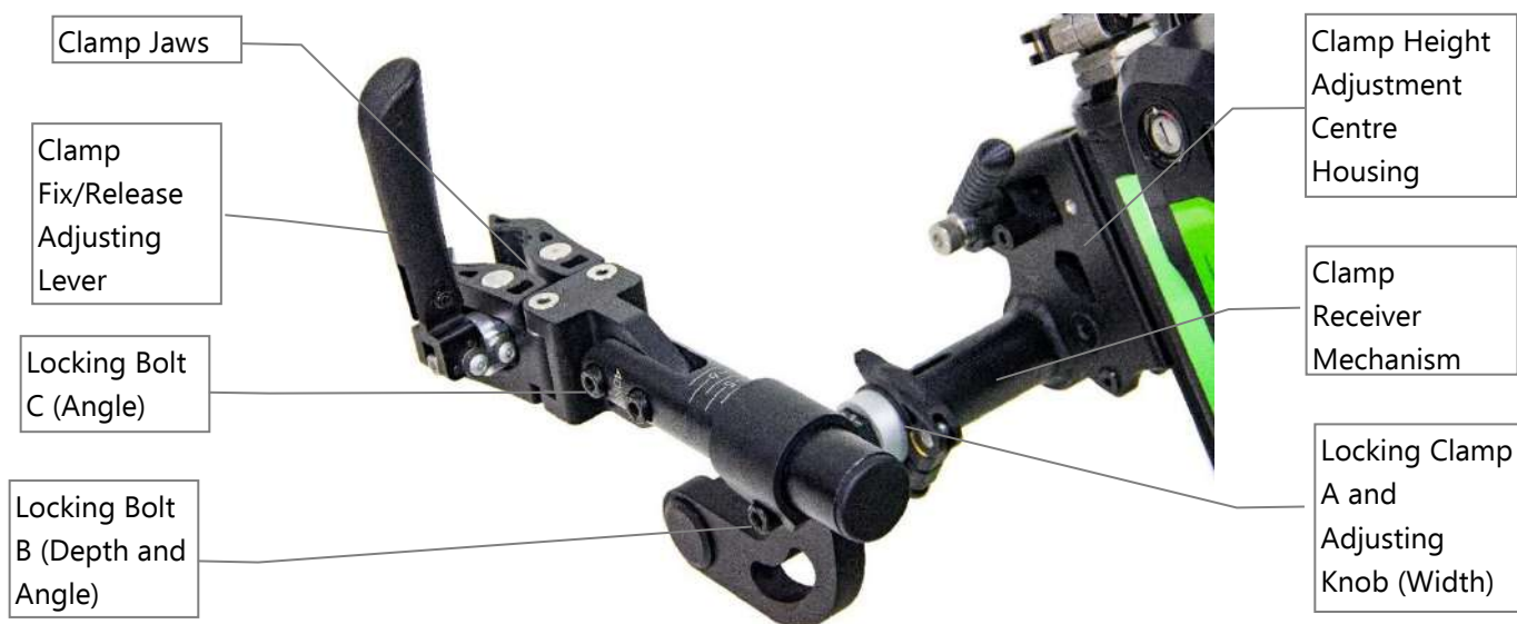
Figure 12. Manual Clamp and Width Adjustment Assemblies
