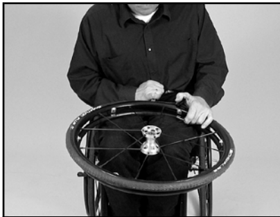
Image 28 Pull the tyre edge over the rim
