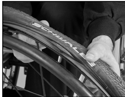
Image 29 Pull out the tube
