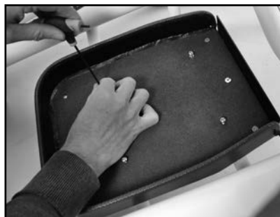
Image 20 Re-attach the footrest
