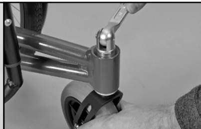
Image 52 Screw the nut off
