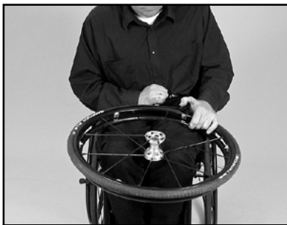
Image 71 Pull the tyre edge over the rim
