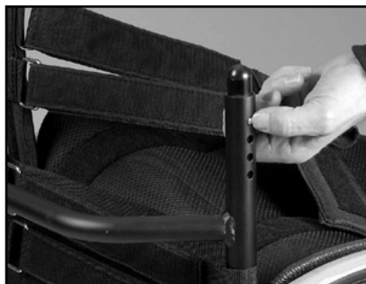
Image 24 Press the spring lock in
